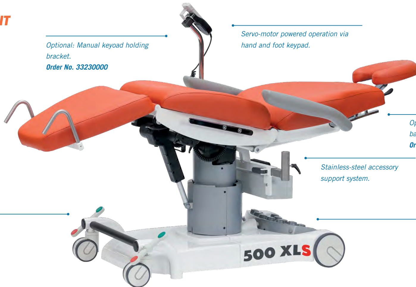
Removable foot keypad for backrest, seat and height adjustment, including on-off button, 3 memory positions, and a reset key.
